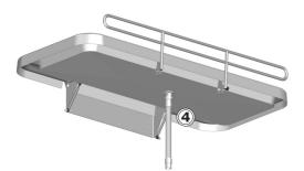
• Check the drain pipe connections ④, and check and clean the water trap (if fitted).
