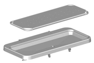
The frame with the cover can be removed for cleaning. It can be zipped off and washed in regular washing machine at max 70° C. Dry the water collection tray.
