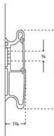
Dimensions for Horizontal Wall Track (side view)
