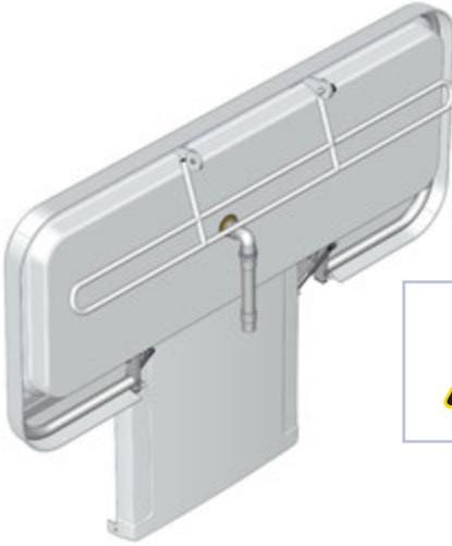
Support the bench using your hand or body when folding it down, to avoid the risk of damage.
