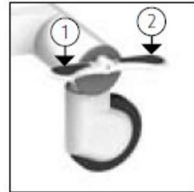
Figure 3 Semi-central braking and moving forward.
